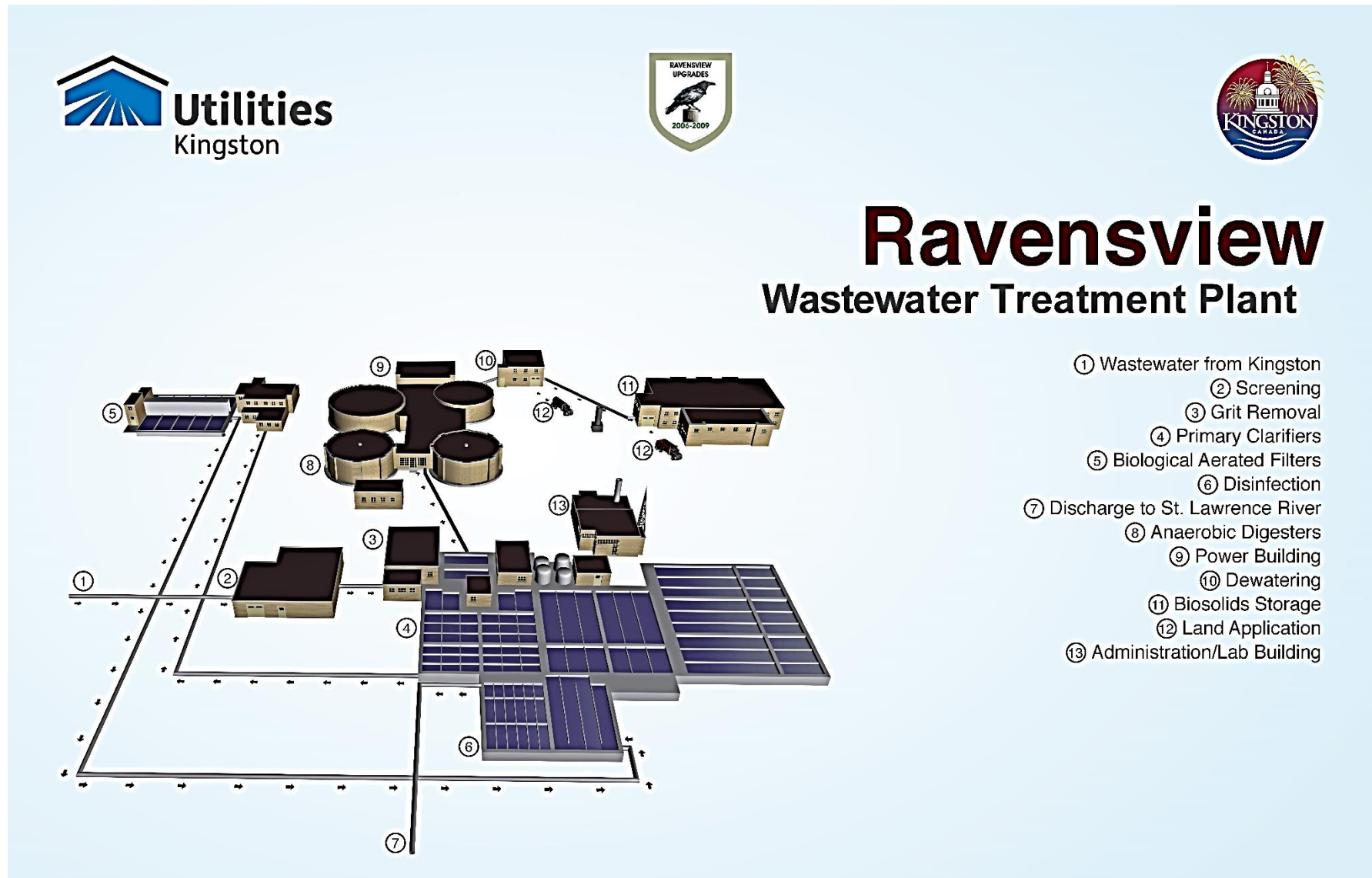
Figure 1 - Ravensview Wastewater Treatment Plant General Layout
