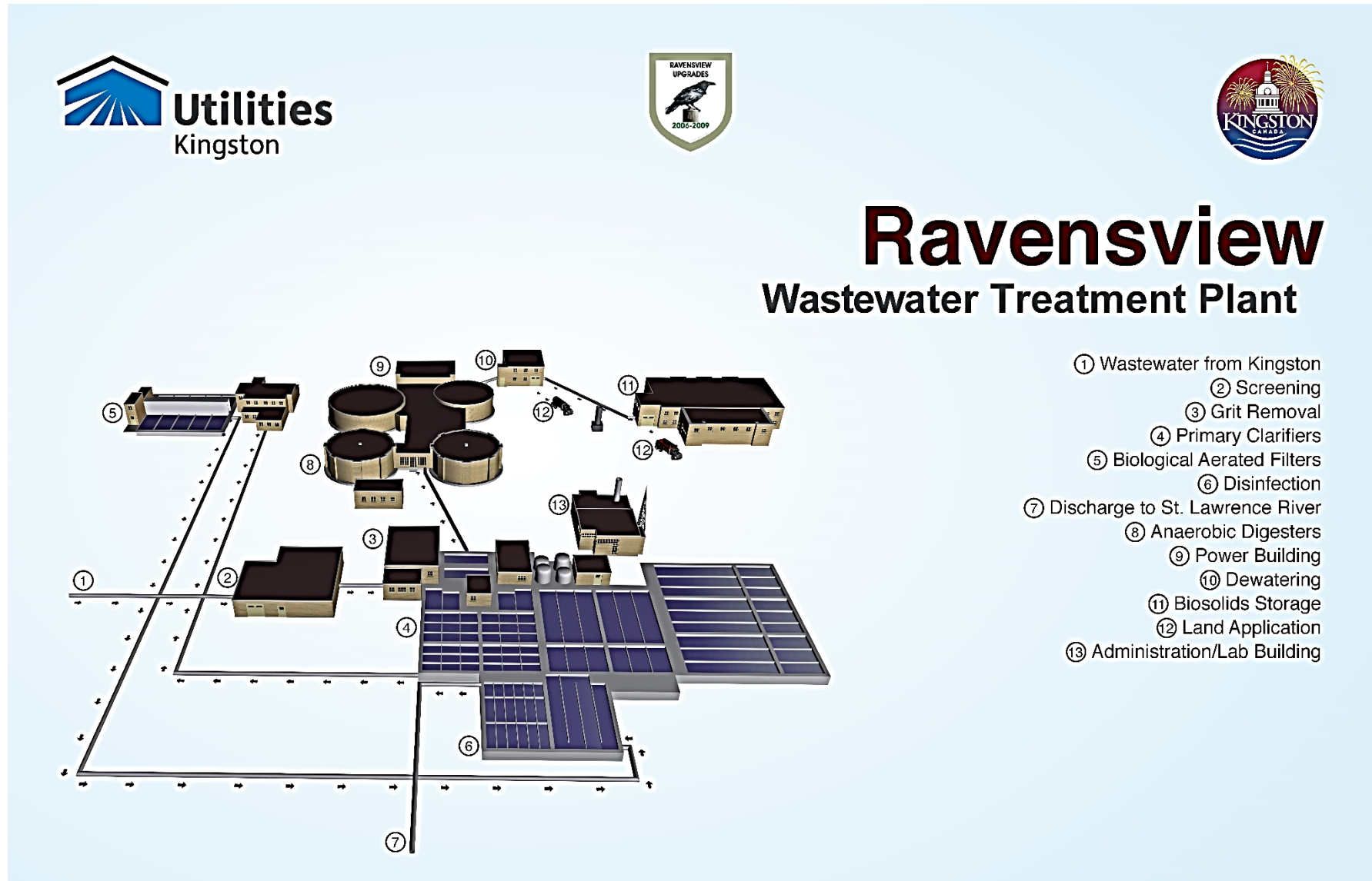
FIGURE 1 - RAVENSVIEW WASTEWATER TREATMENT PLANT GENERAL LAYOUT
